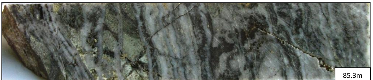
Figure 28. ADH 002 coarse chalcopyrite in a quartz veined andesite (81.8m).
