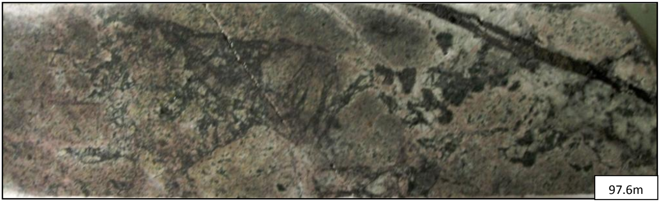
Figure 31. ADH 002 brecciated and weakly potassically altered microdiorite with magnetite veinlets.
