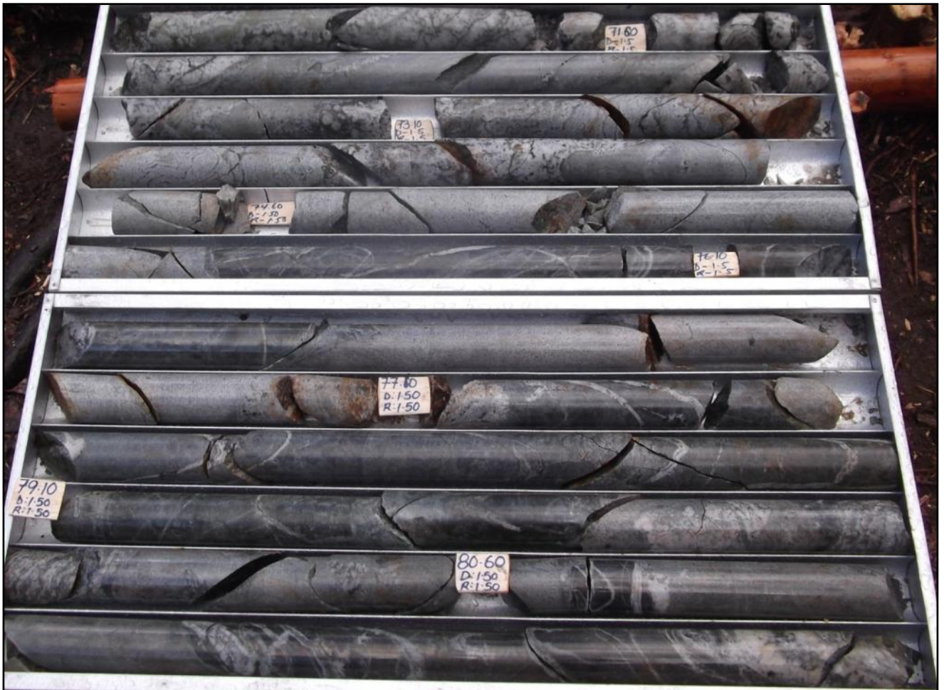
Figure 36. ADH 002 propylitically altered andesite with cross cutting potassic alteration - K-spar veining.
