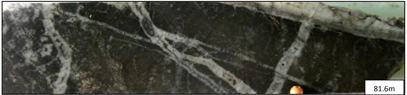
Figure 27. ADH 002 quartz, pyrite, chalcopyrite filled fractures in andesite (81.6m).
