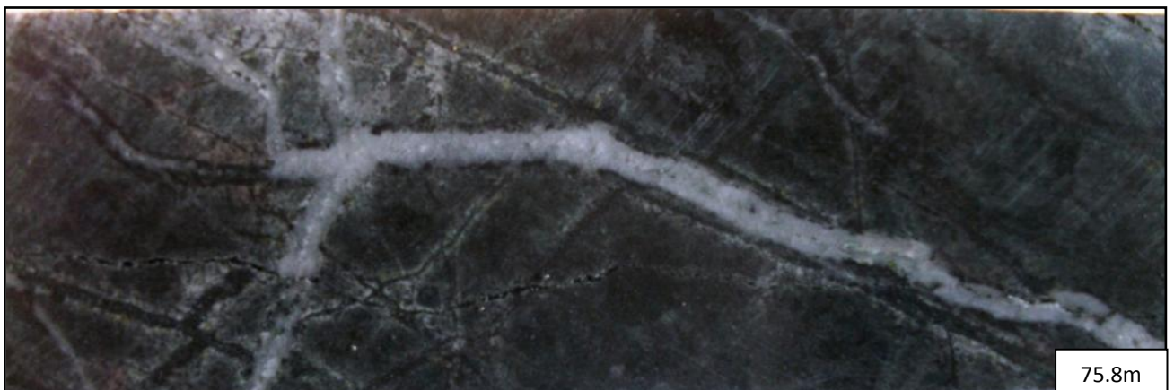
Figure 26. Quartz, pyrite, chalcopyrite filled fractures in andesite (75.8m).
