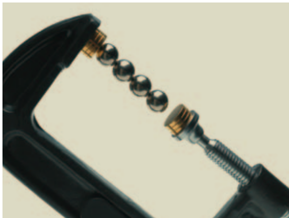
Figure 3: (left) Six neodymium rare-earth magnets suspend four 5/8 inch diameter steel balls (right) the Millan Valley Bridge in France
