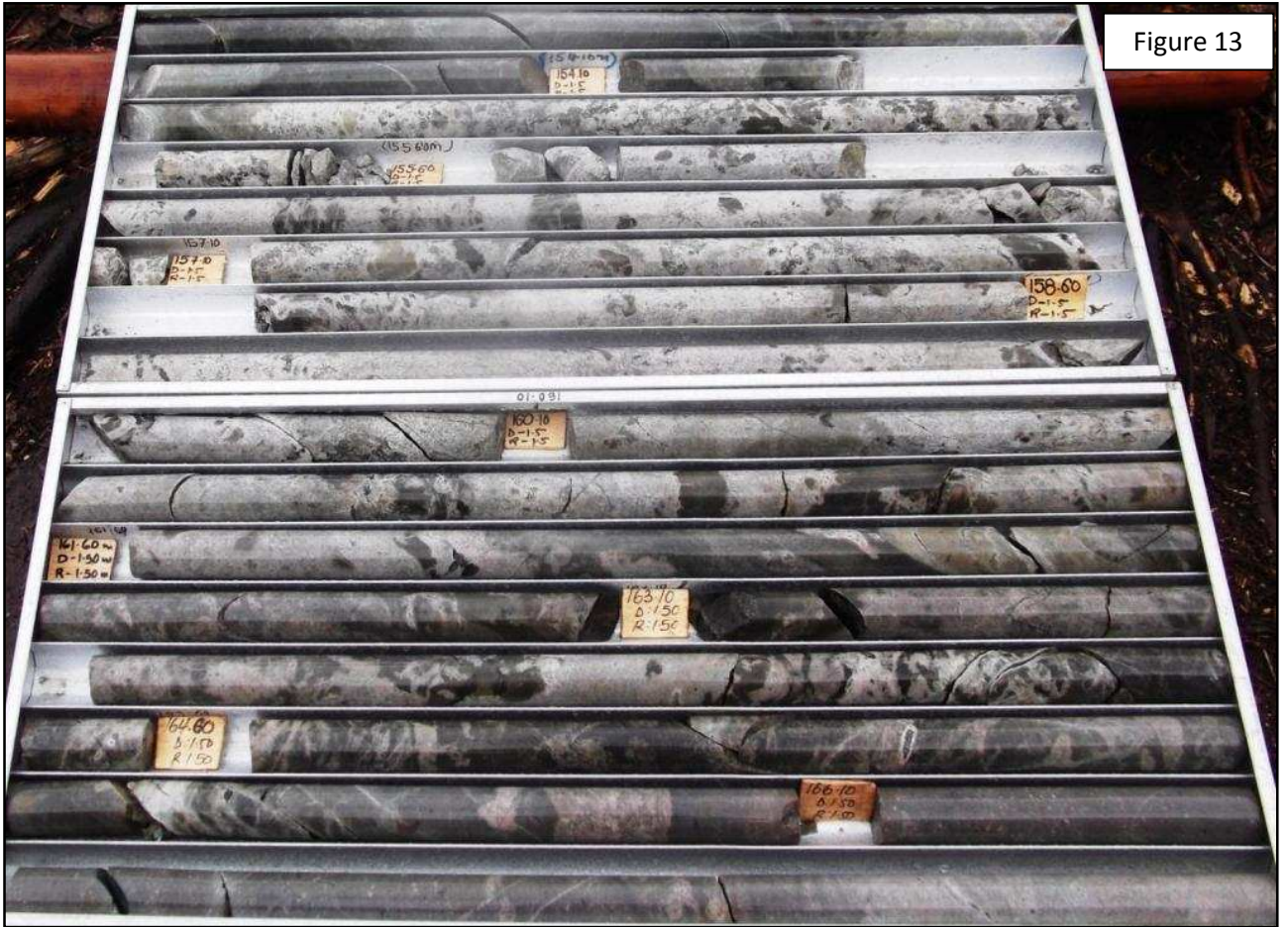
Figure 13. Hole ADH 002 whole drill core from 152.6m to 167.4m downhole, showing most of the 19m intercept grading 1.86g/t gold + 0.18% copper.
