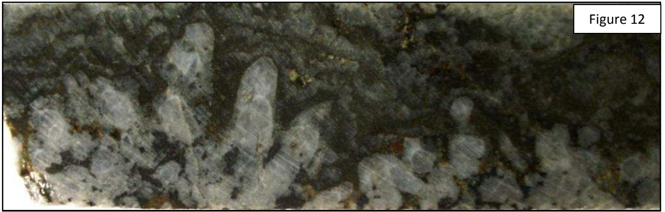
Figure 12. Radiating quartz crystals with fine grained pyrite and chalcopyrite. Open space growth is noted (70.1m) with the 1m sample grading 0.87% copper + 0.60 g/t gold + 126 ppm molybdenum.
