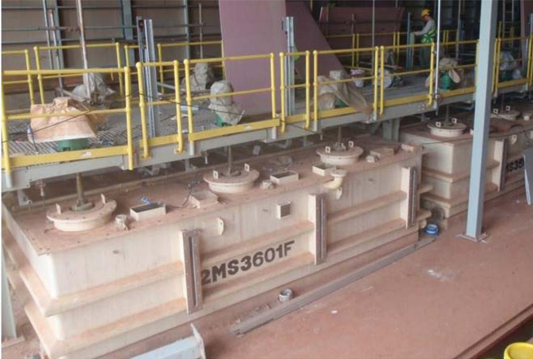
**Post Treatment Workshop: Precipitation Tanks and Centrifuges**
