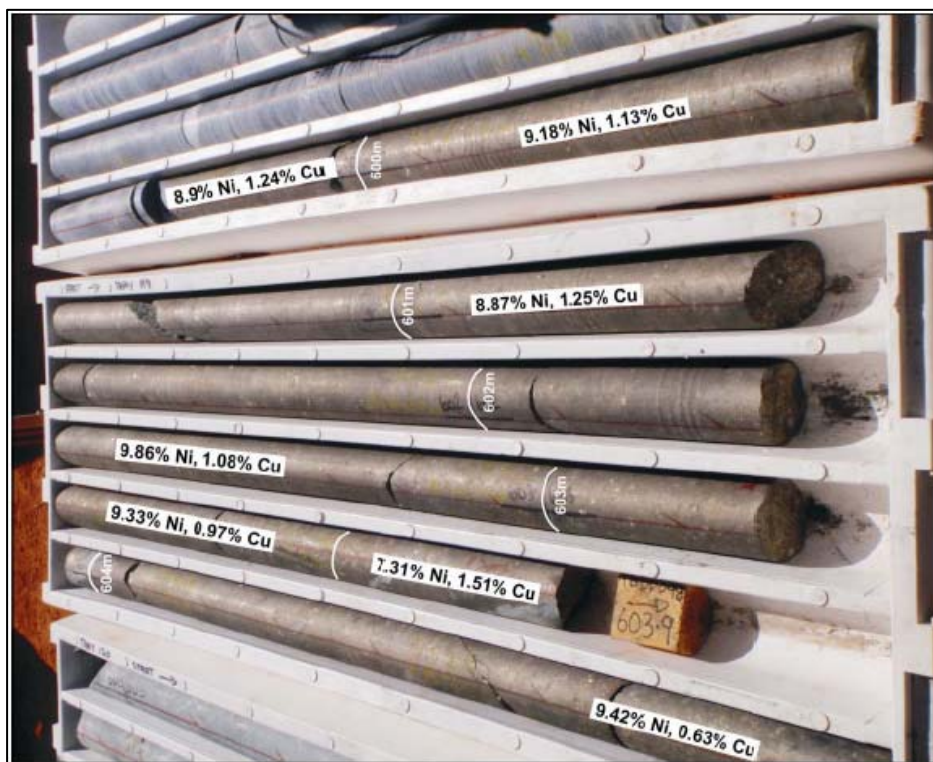
Figure 4 – Duketon Nickel JV Rosie Prospect - TBDD098 Massive sulphide intercept - 5.20m @ 9.13% Ni, 1.09% Cu, 0.21% Co and 7.09g/t PGEs (PGEs include 2.22g/t Pt, 1.74g/t Pd, 0.82g/t Rh, 1.79g/t Ru).
