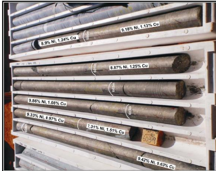
Figure 7 – Duketon Nickel JV Rosie Prospect - TBDD098 Massive sulphide intercept - 5.20m @ 9.13% Ni, 1.09% Cu, 0.21% Co and 7.09g/t PGEs (PGEs include 2.22g/t Pt, 1.74g/t Pd, 0.82g/t Rh, 1.79g/t Ru).
