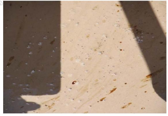
Return mud-stream Surprise-1 showing free gas breakout and oil slicks in 8.9 ppg/1.07 SG mud (slightly overweight)-viewed on circulation after electric logging runs before planned check shot survey. Gas composition C1/C2/C4/C5 percentages 41 /24/ 20/ 11/ 4 respectively. Note : No conclusions can be definitively made on the capability of the well to flow oil to surface from these indications but they are regarded as positive indicators rather than negative indicators.
