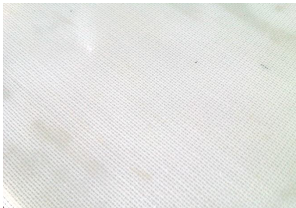
Figure 3 (left) – A close-up shot of the GE anion exchange membrane Figure 4 (right) – Membranes cut to size prior to being inserted into the pilot cell
