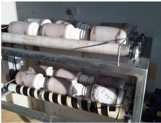
Figure 1 (left) – Bottle roll testwork on Barnes Hill saprolite samples Figure 2 (right) – 30kg atmospheric vat leach testwork
