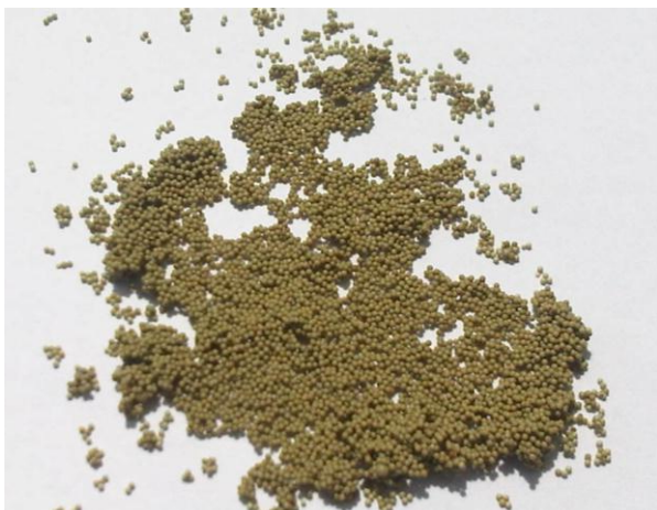
Figure 6 (left) – Dow Chemical selective nickel low-pH Ion Exchange resin Figure 7 (right) – The new cell designed for the Barnes Hill flowsheet moving into position
