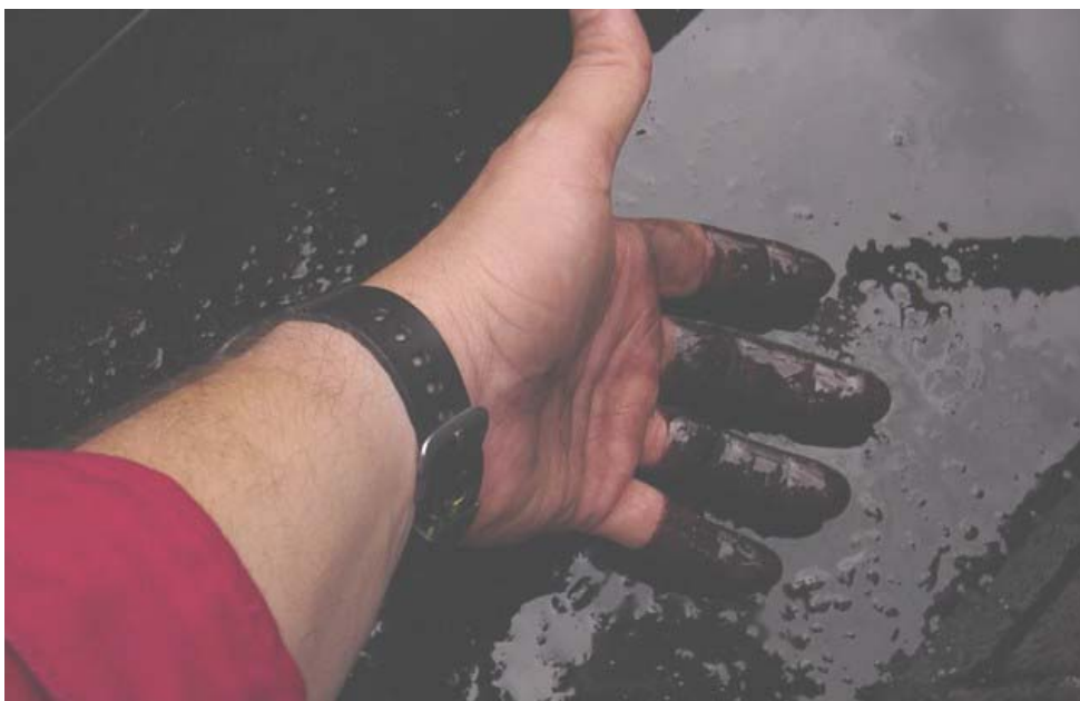
Oil on the surface of drilling fluid in the possum belly -Note: As the oil is floating on the surface of the drilling fluid and dispersed in droplets throughout, no quantification of oil volumes can be given.
