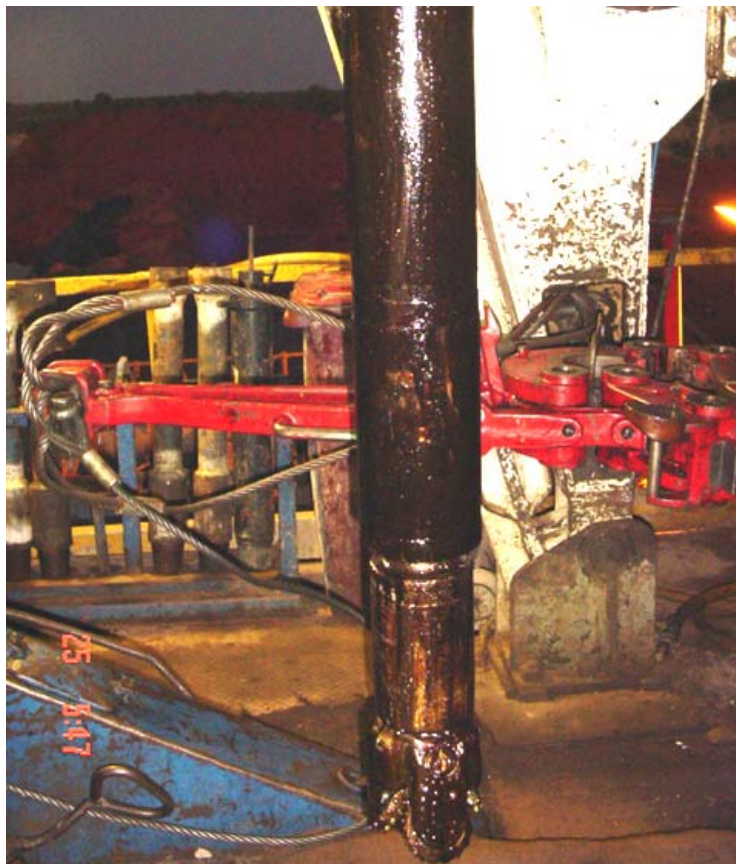
Oil coating 6" drill bit during horizontal drilling operations.
