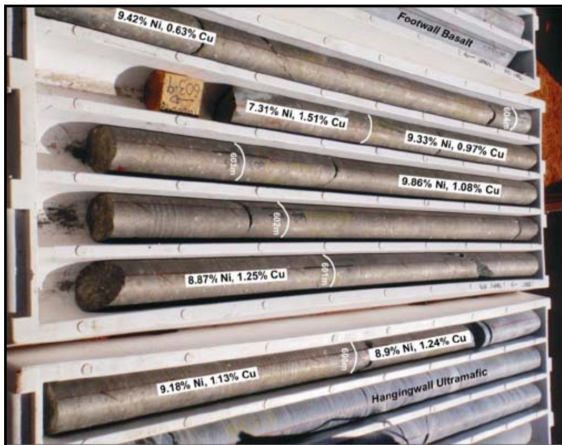
Figure 8: Rosie deposit massive sulphides in TBDD098, with coarse grained pentlandite porphyroblasts. The down hole intercept comprised: 5.20m @ 9.13% Ni, 1.09% Cu, 0.21% Co and 7.09g/t PGEs (PGEs include 2.22g/t Pt, 1.74g/t Pd, 0.82g/t Rh, 1.79g/t Ru).
