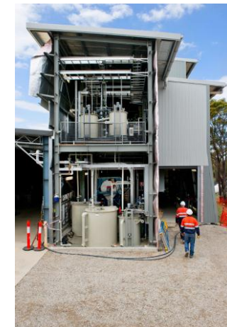
Sulphation & Purification Demonstration Plant 2012 ANSTO, Sydney
