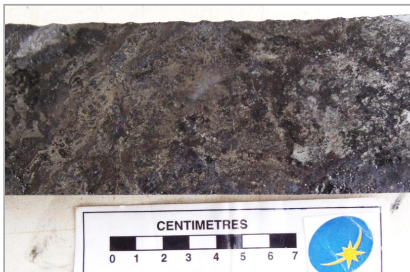
Photo: PPDH 2 half core at 66.3 metres – a massive sulphide segment of the very high grade intersection from 66m to 67m. Random handheld XRF analyses from the photograph area returned values of 1.0% to 3.9% silver consistent with the laboratory assay of 2.25% silver for the full one metre sample submitted for the other half of the core.
