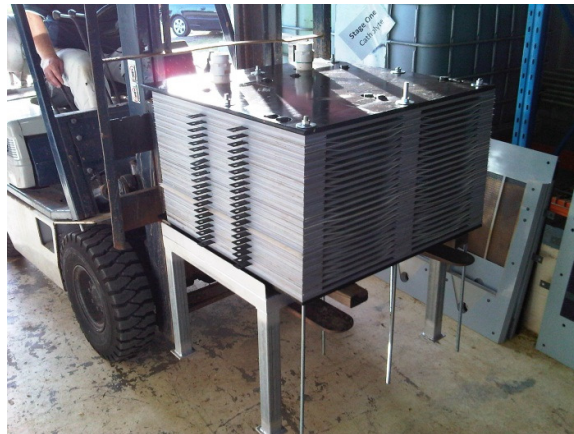
Figure 6 – The new cell designed for the Barnes Hill flowsheet moving into position
