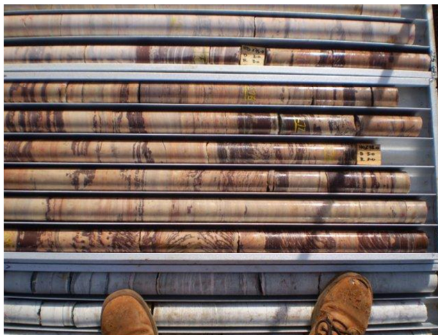
Figure 2 – Tray 36 Intersecting the Sandstone Unit at Lindeman’s Bore
