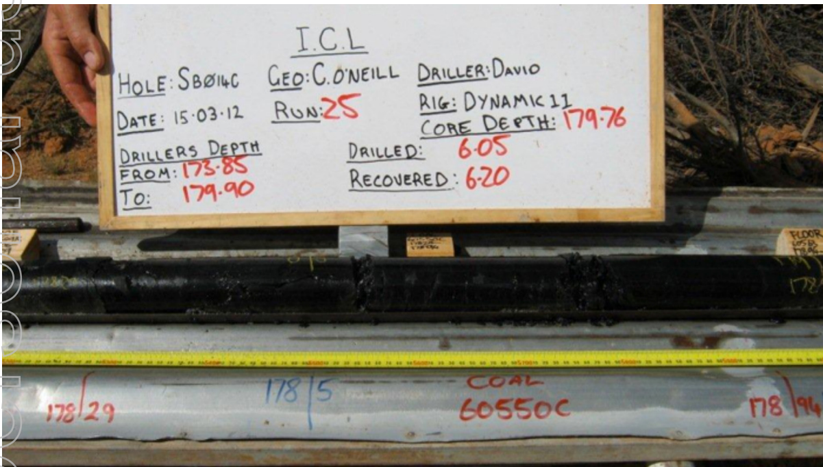
Coal intersect from SB014C at EPC 2197 – Core sample taken from diamond drilling
