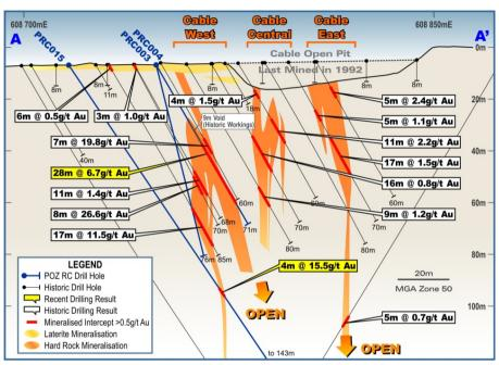
Cable East Vein is a continuous 500m long mineralised structure
