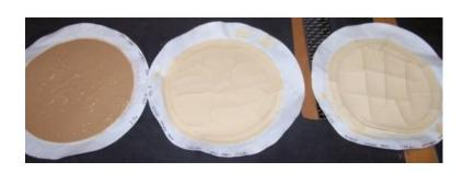
POZ Products from fines WHIMS testing. Iron rich residue on left. Samples to right are the non-magnetic fractions (phosphate rich)
