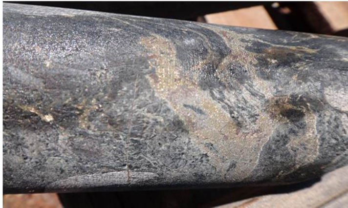
Figure 4 – Minor pyrite and chalcopyrite stringer development in a foliated and banded, hematite/magnetite/chlorite meta-sedimentary rock unit at 423.6m
