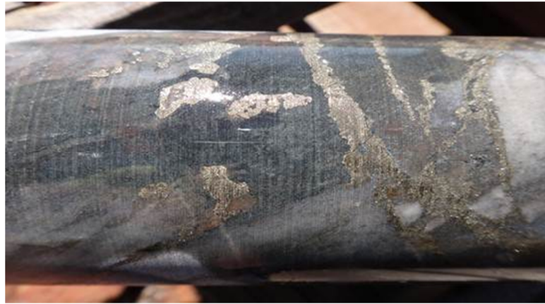
Figure 2 –Pyrite and chalcopyrite in stingers and on joint planes in black shale rock at 415.4m
