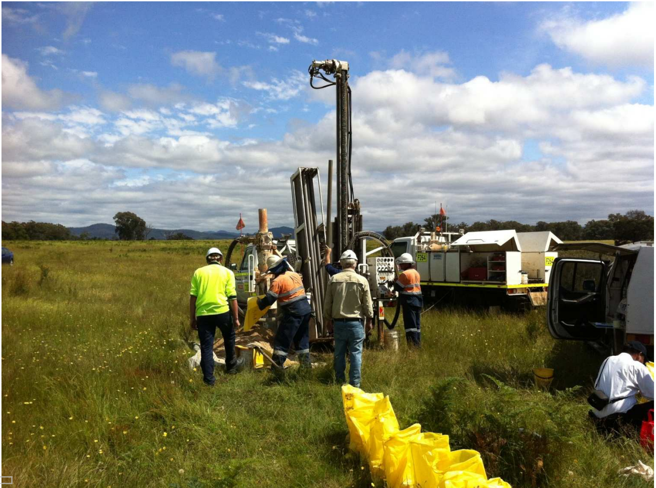
Figure 7: Low impact aircore drilling in the central portion of the Glenaladale area (December 2011)
