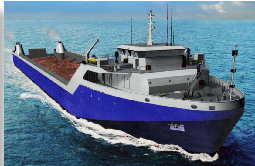
Feeder barge carries ore to floating harbour
