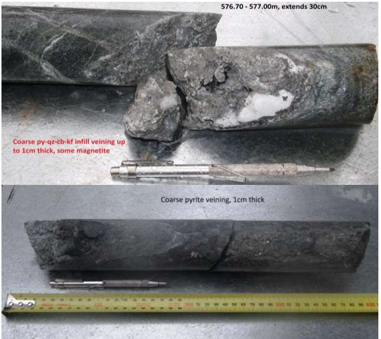
Photo 1a and b: Vein extends up to 30cm and infill with semi-massive coarse pyrite (>10%) grains and quartz, k-feldspar and carbonate, range between 576.70 – 577.60m.
