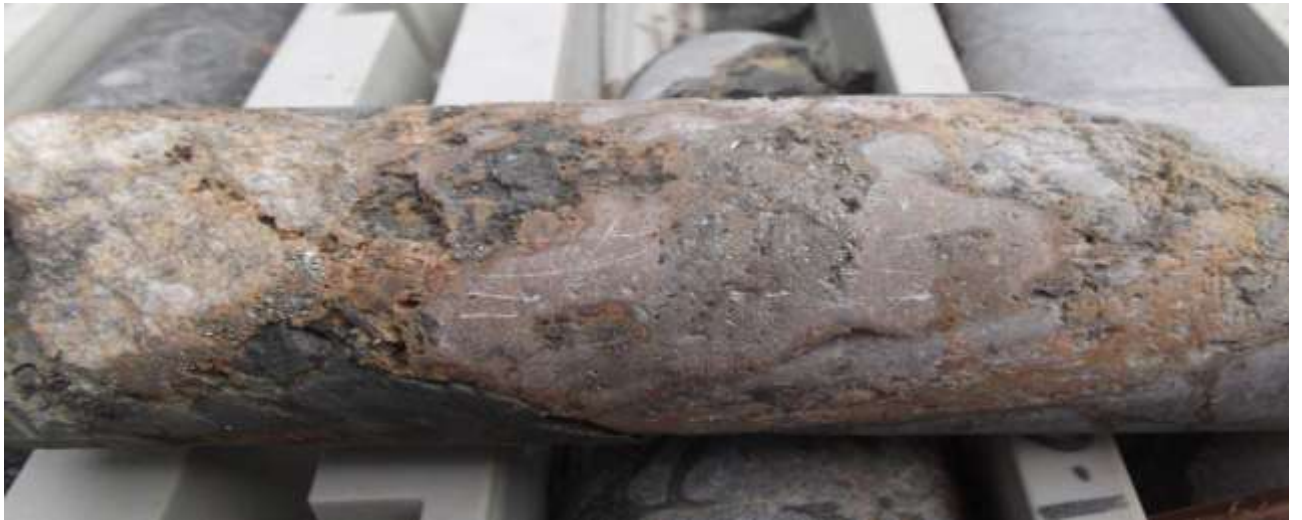
Photo 4: Quartz- pyrite-kfeldspar/siderite? breccia band from 360.90-361.10m . Notice the pyrite bleb in the centre of image and orange yellow k-feldspar (?) and or siderite?
