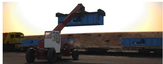
Figure 2: Loading of sealed containers at the Cloncurry Multi-user Rail-load Facility - 3D design model
