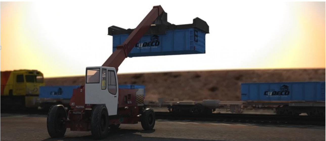
Figure 3: Loading of sealed containers at the Cloncurry Multi-user Rail-load Facility - 3D design model
