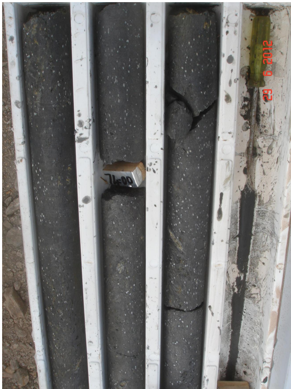
Plate 3. HQ drill core of highly graphitic schist in hole CSDD12_003
