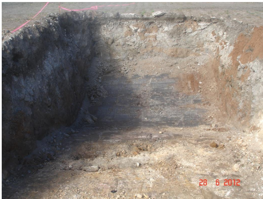
Plate 4. Drill sump prepared for diamond drill hole CSDD12_003 showing thin overburden overlying intense graphite mineralisation.
