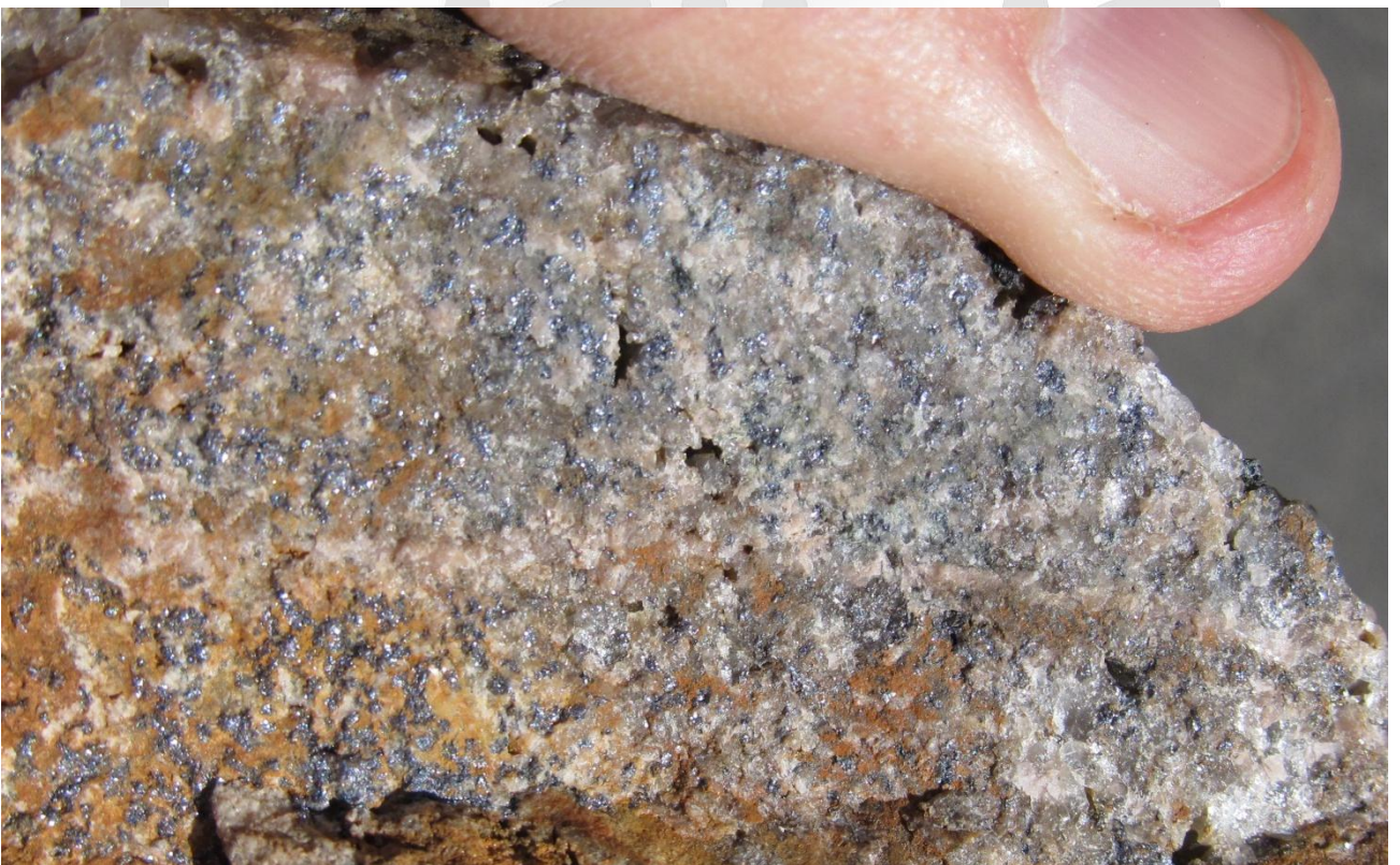
Figure 11. Surface rock sample with molybdenite (molybdenum sulphide - silver grey coloured) around quartz-K feldspar veinlet in strongly silicified quartz monzonite porphyry.
