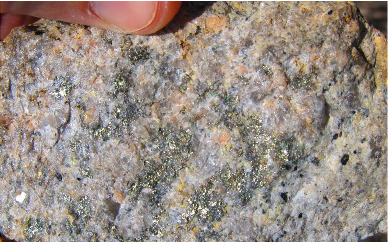
Figure 10. Surface rock sample with copper minerals chalcopyrite (brassy yellow), bornite (purplish/bluish silver) and small specks of malachite (green) in potassically altered quartz monzonite porphyry.
