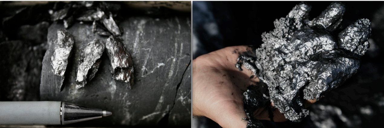
Figure 3. Selected examples of graphite mineralisation intersected during drilling, Nunasvaara.
