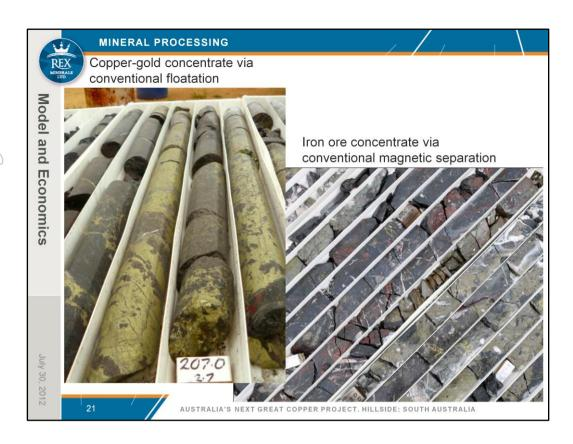
Mineral processing is first by conventional floatation to produce a copper-gold concentrate and the tailings is then treated using conventional magnetic separation methods to produce an iron-ore concentrate.
