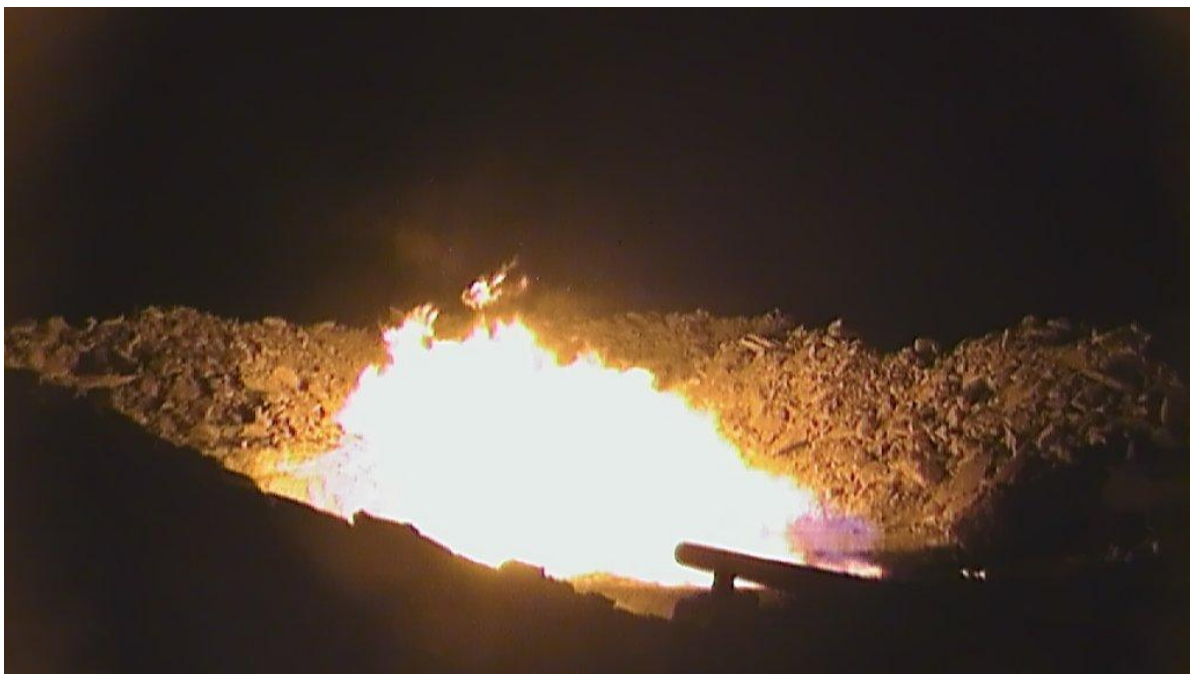
Figure 1: Gas Flare during Testing at Glyde #1 Lateral Well Measured Well Depth of circa 670m
