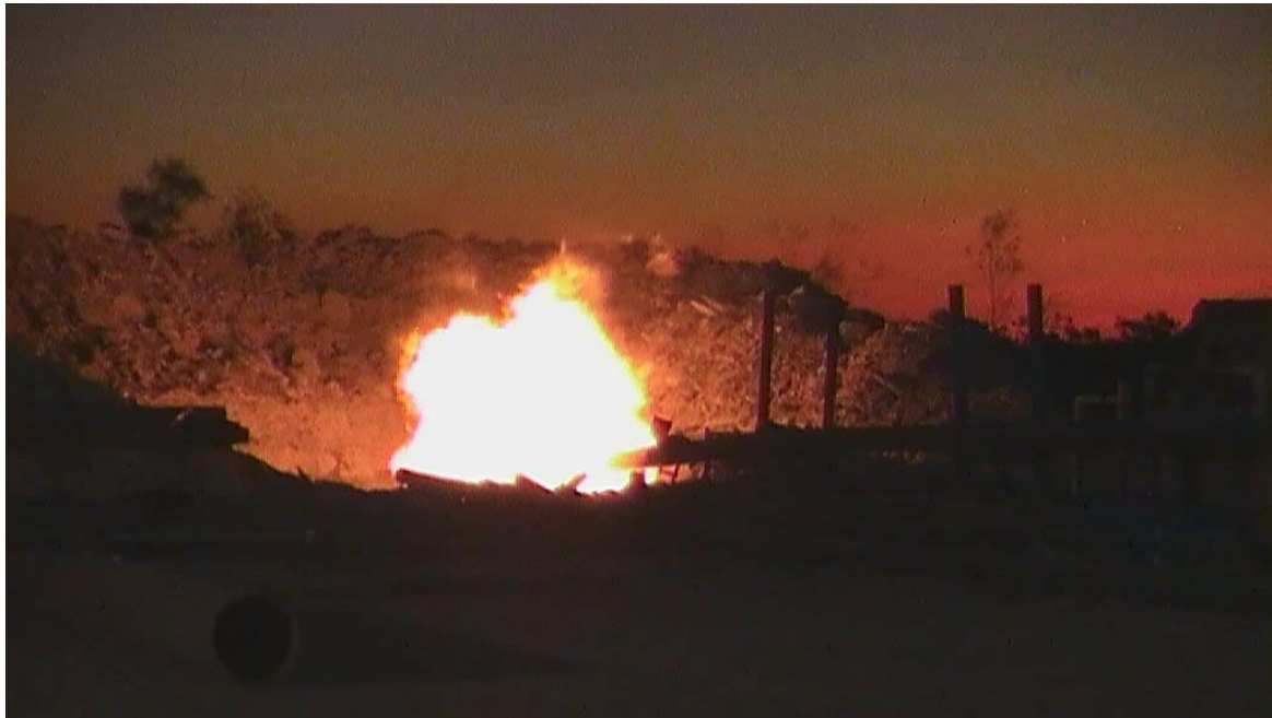
Figure 3: Gas Flare during Drilling with Compressed Air at Glyde #1 Lateral Well Measured Well Depth of circa 770m
