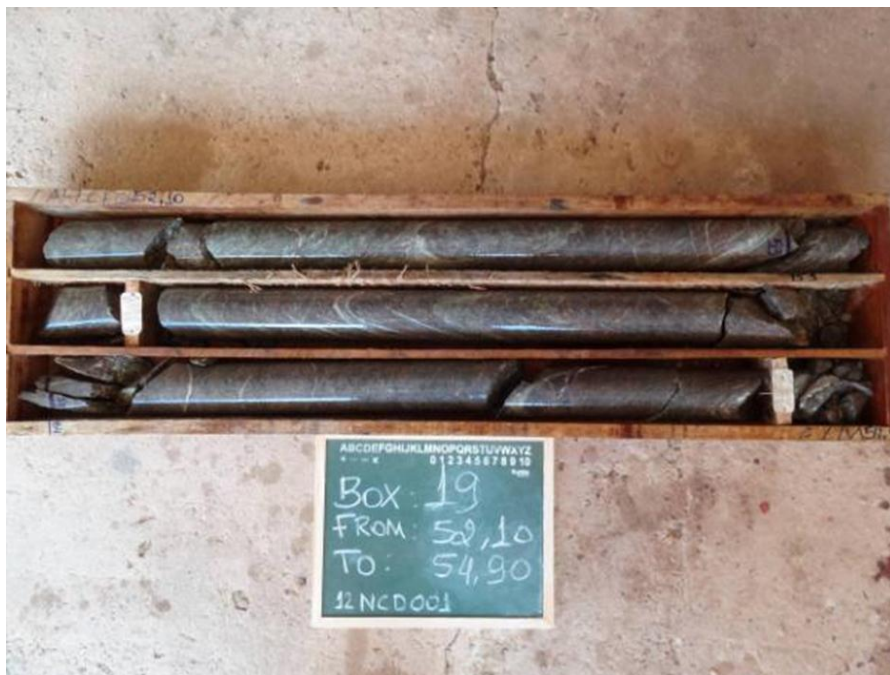
Figure 5 – Altered sheared granite 12NCD001
