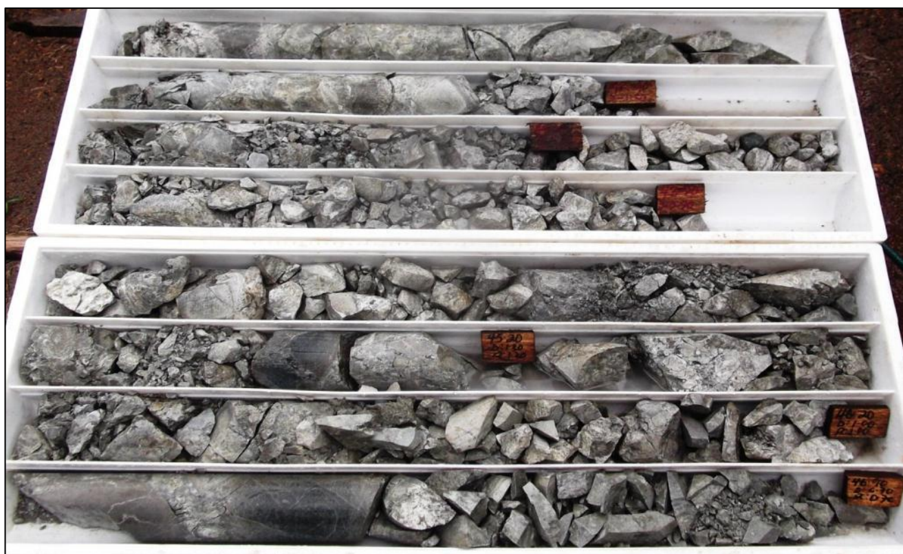
40.9 – 46.9m: Quartz Andesite Breccia unit – cracked, strongly silicified and argillic altered enriched w/white puggy clay material.
