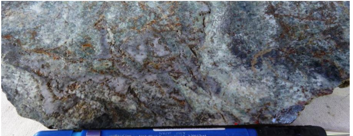
qz-chl-fuchsite-k feldspar/hem breccia in fracture Zone, part of 1-2m breccia.
