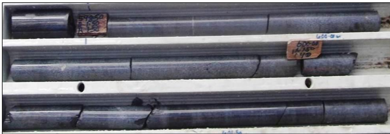
Weakly mineralised and altered microdiorite at 598-600m
