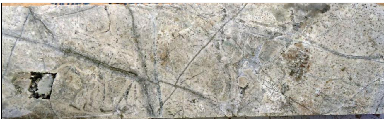
Brecciated bleached rock with late qz-py-sulph veins@463.00m – 463.30m
