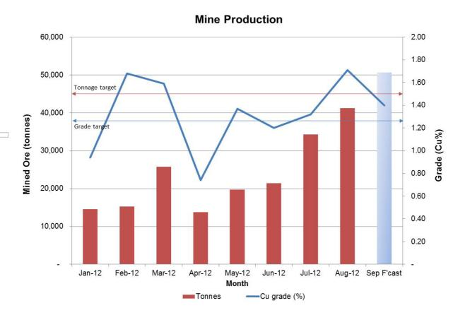
Ore production commenced in January 2012 from ore in development drives. Stoping commenced in late May and production volumes are increasing such that they are now approaching design rates of 550,000 tonnes per annum (46,000 tonnes per month). Grades are predicted to average 1.3% copper for the 2012/2013 year and 1.5% copper for the life of mine but are currently exceeding 1.5%.
