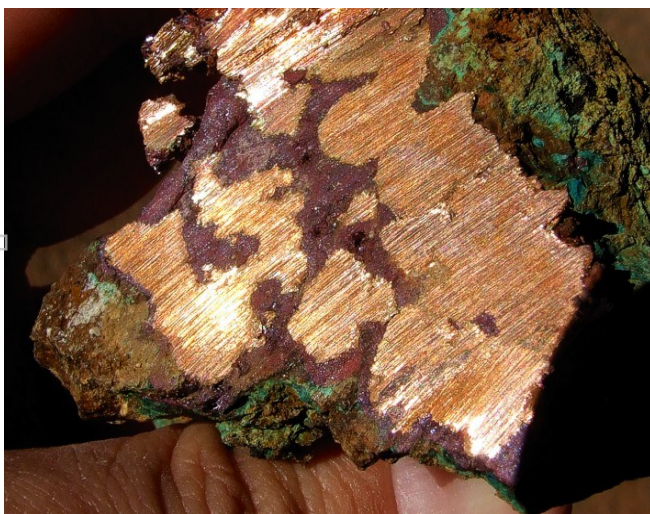
Figure 13: Native copper nugget cut with diamond saw, recovered at 5m depth from test costean excavated earlier in the year over Las Minerale. The area defined as the “native copper domain” within the current resource block model, did not identify native copper to be present at the depths being targeted in the deep costean.
