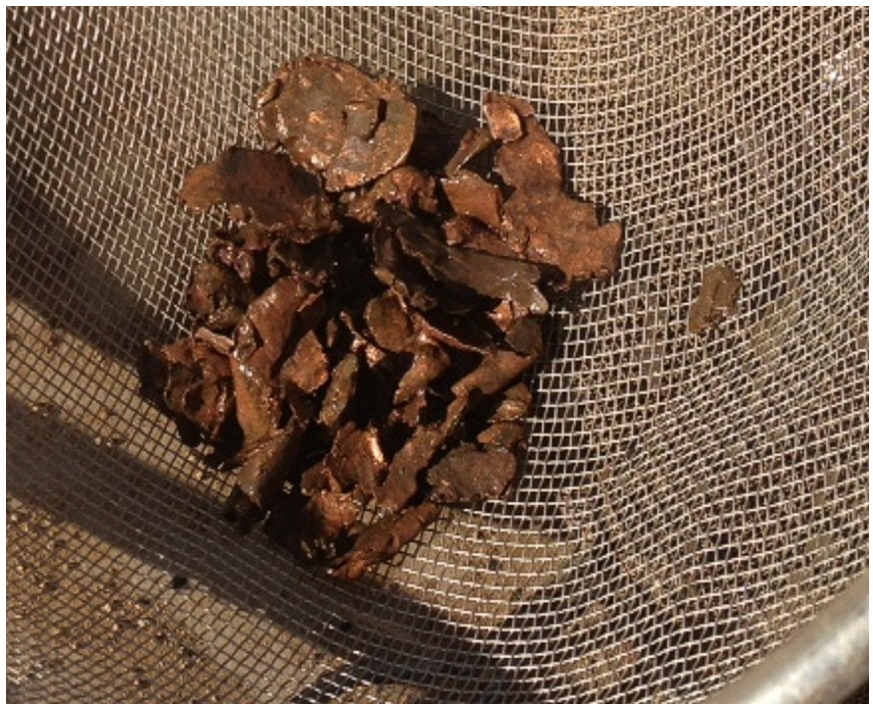
Figure 18: Native copper flattened by the bedrock drill, recovered from LMOX703, from 18-25m, in an area not previously identified to host native copper. Many of the pieces are larger than 20mm in size.
