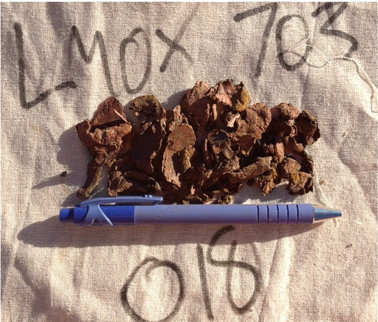
Figure 11: Native copper flattened by the bedrock drill, recovered from LMOX703, from 18-25m, in an area not previously identified to host native copper.
