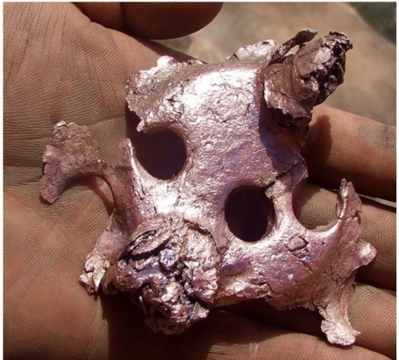
Figure 17: Example of large native copper nugget, possibly encountered in soft clay or friable oxide material and unable to return up the small (20mm) sample return holes at the end of the RC bit. Left; the remaining middle section appears to have been "stamped" out of a larger solid copper nugget that has been flattened, then cut through by the bit and right; underside of the copper "stamp" showing how the metal was pushed into the two 20mm sample return holes (top right & bottom left) and was unable to return to surface
