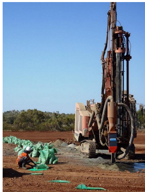
Figure 20: The green-grey/olive coloured high-grade copper-rich ore is easily identified against the red-coloured, iron-rich gangue (waste) material left on surface after completion of the bedrock holes.
