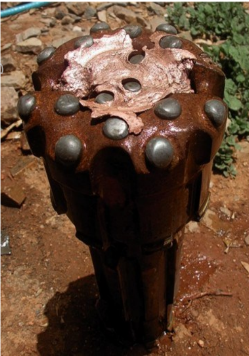
Figure 17: Example of large native copper nugget, possibly encountered in soft clay or friable oxide material and unable to return up the small (20mm) sample return holes at the end of the RC bit. Left; the remaining middle section appears to have been "stamped" out of a larger solid copper nugget that has been flattened, then cut through by the bit and right; underside of the copper "stamp" showing how the metal was pushed into the two 20mm sample return holes (top right & bottom left) and was unable to return to surface
