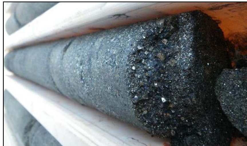
Drill core showing supergene chalcocite with copper grades up to 45%
