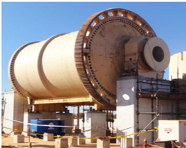
Ball Mill Installed On Plinths
