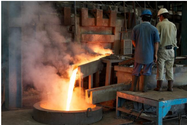
Figure 6 & 7: Tapping of molten tin from the smelter and vat pouring ready for continuous casting of ingot
