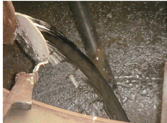
Figure 6 & 7: Tapping of molten tin from the smelter and vat pouring ready for continuous casting of ingot
