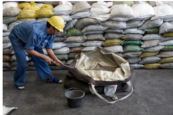
Figure 4 & 5: Tin Concentrate and Sampling for analysis prior to smelting operations
