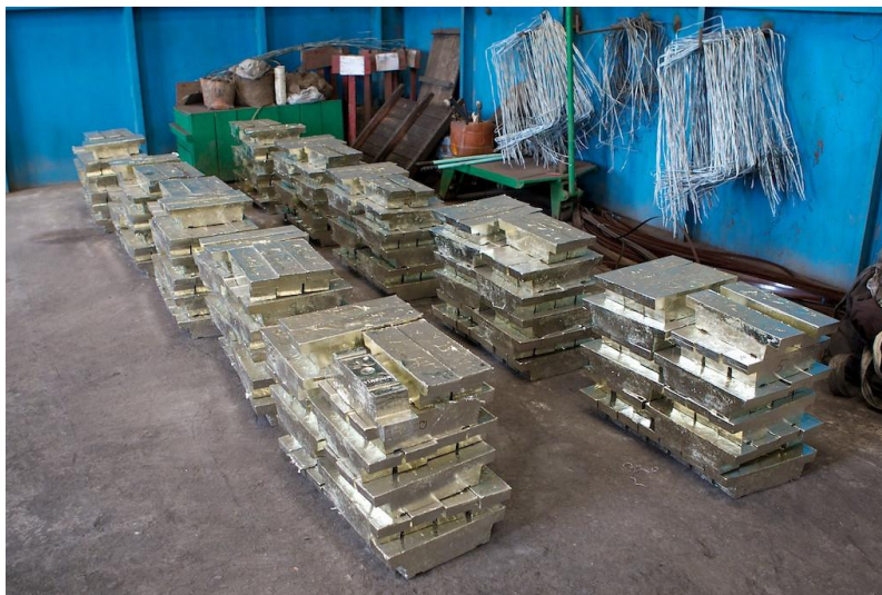
Figure 8: Ready LME Grade A (<50ppm Pb) 25 kg tin ingots ready to pack and ship to markets from Yinchen smelting facility
