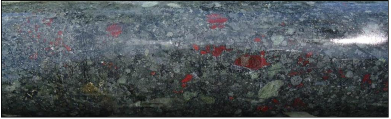
Abundant hematite blebs in a brecciated pyroxene andesite unit at 432.20m – 432.40m
