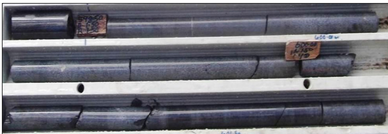
Weakly mineralised and altered microdiorite at 598-600m
