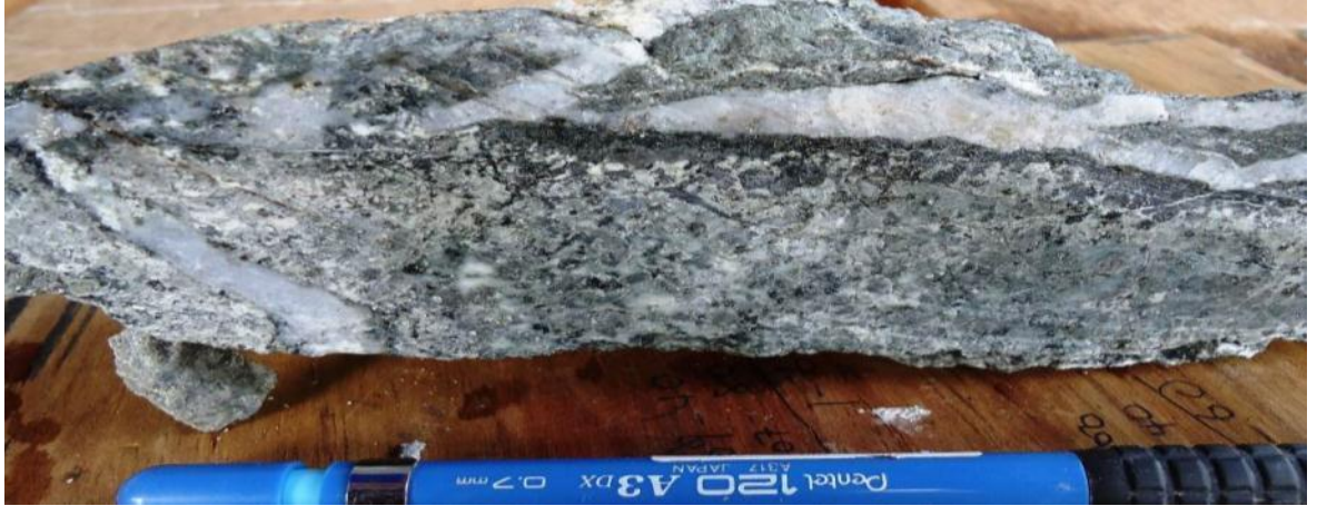
qz-cb-mo vein in a cly shear. Notice Moly rimming vein
