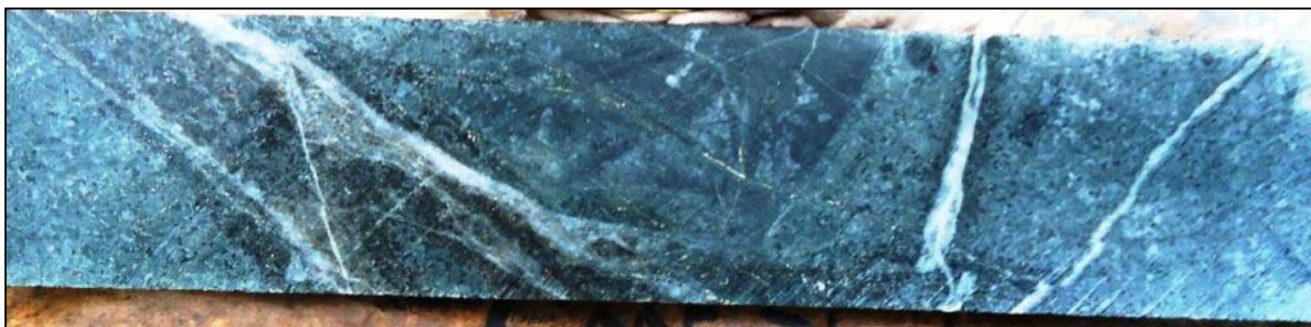
Host rock Pyroxene Andesite, variably brecciated with sheeted qz-carbonate veins @670-670.30m
