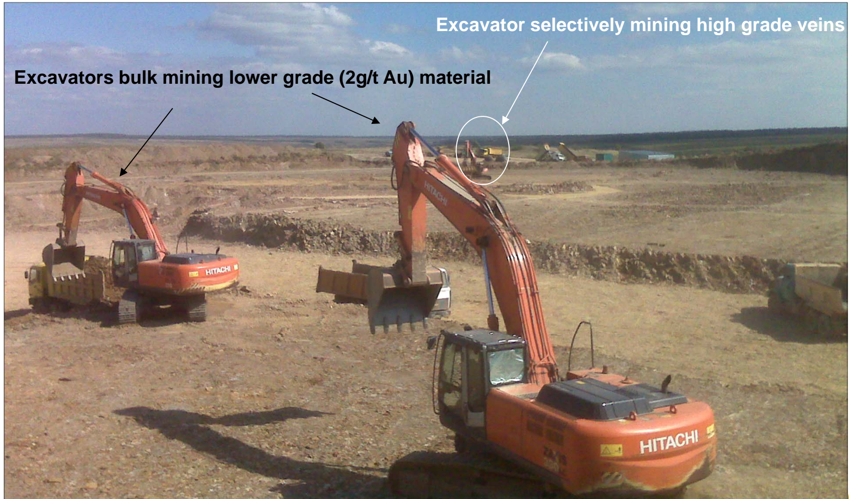
Selective mining. In the background excavator mines high grade veins averaging 8 g/t Au. In the foreground two excavators bulk mine lower grade rock.
