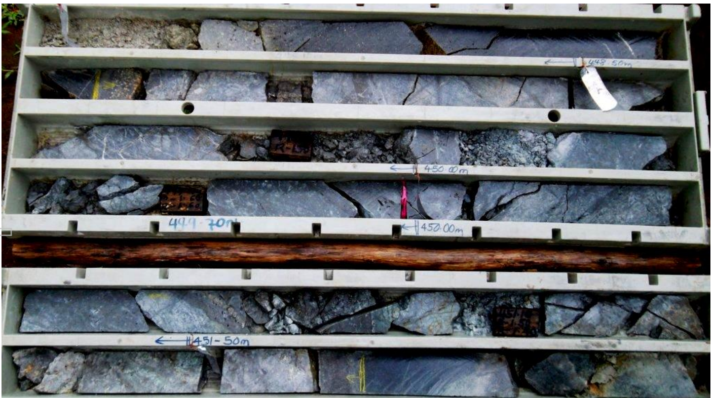
Photo 1 Trays showing core from the high grade zone in ADH013 that has been cut longitudinally for sampling by a diamond bladed cut-off saw. Photos 2-5 follow and are self explanatory.
