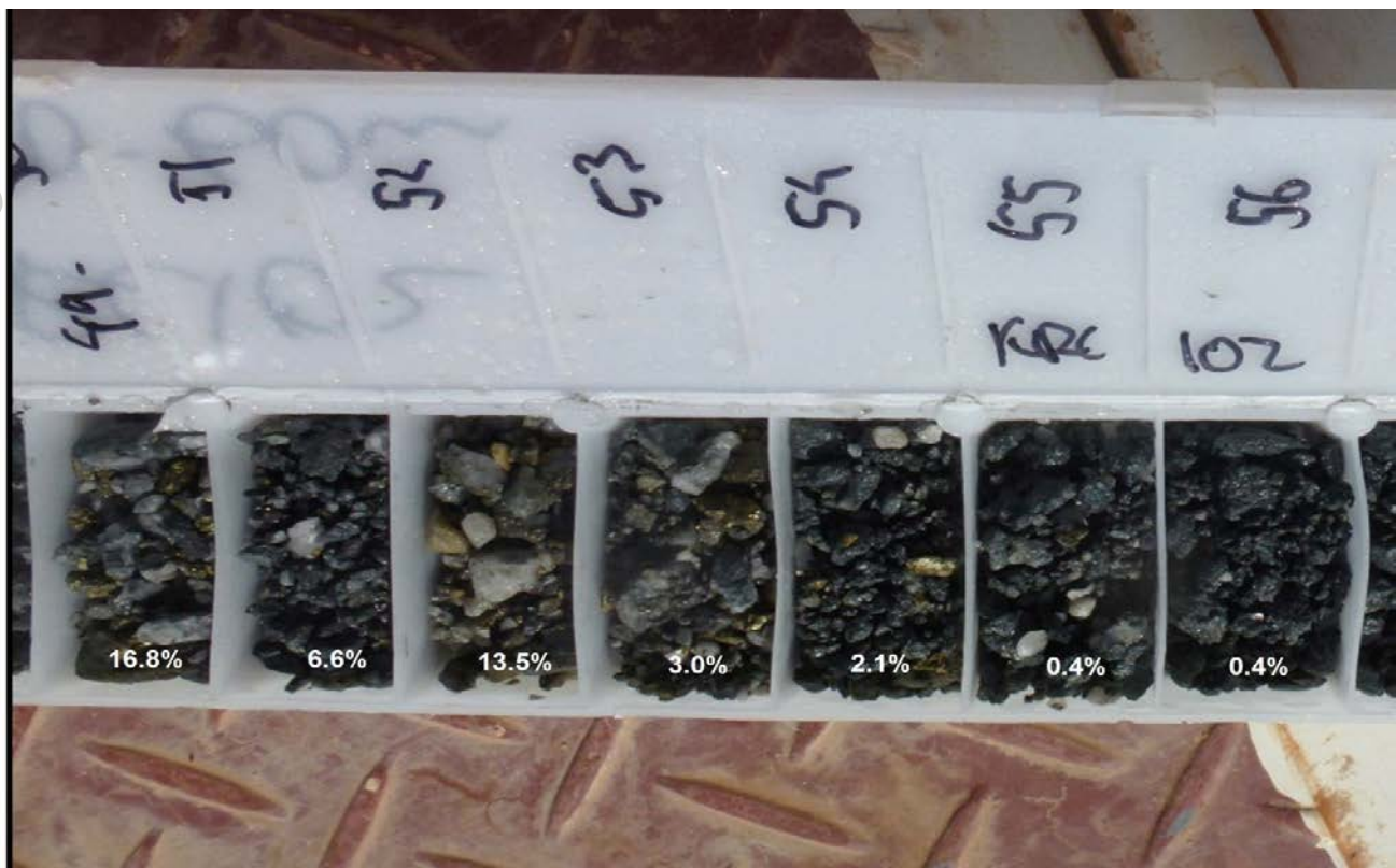
Plate 1 - Drill Chips from KRC102 (49m -56m) showing Copper Grades.
