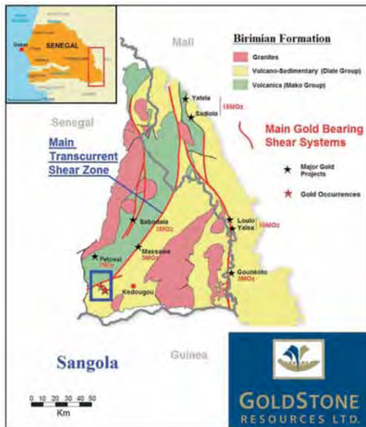
The Sangola permit area lies along the Main Transcurrent Shear Zone which also controlled the formation of the Massawa gold deposit and covers the prospective basalts and andesites of the Mako Group which host the Sabodala and Petowal gold deposits. Exploration in the area depicted on the map resulted in the discovery of more than 30 Moz of gold. The Sangola permit area still holds the potential for new significant gold discoveries
