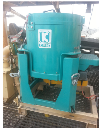
Figures 3 - New leaching tanks and Knelson Concentrator
