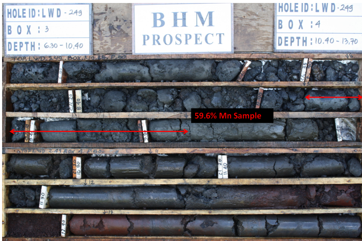
Figure 1: Core tray containing record high-grade manganese assay
