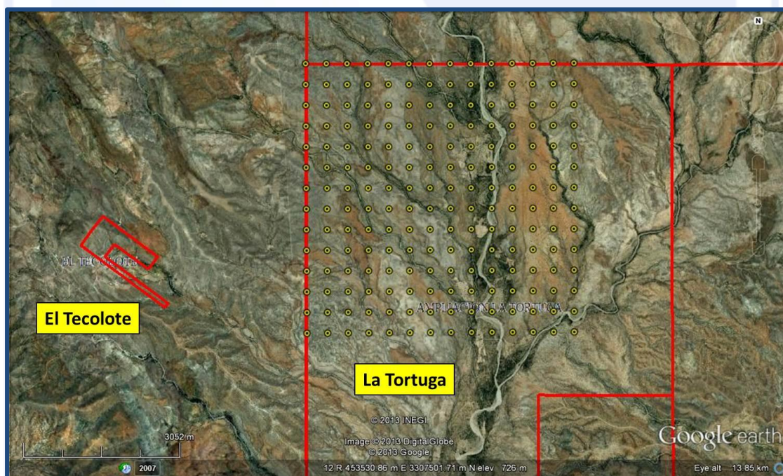
Figure 1: Gravity stations (yellow dots) over Google Earth satellite image showing internal tenement boundaries (in red).
