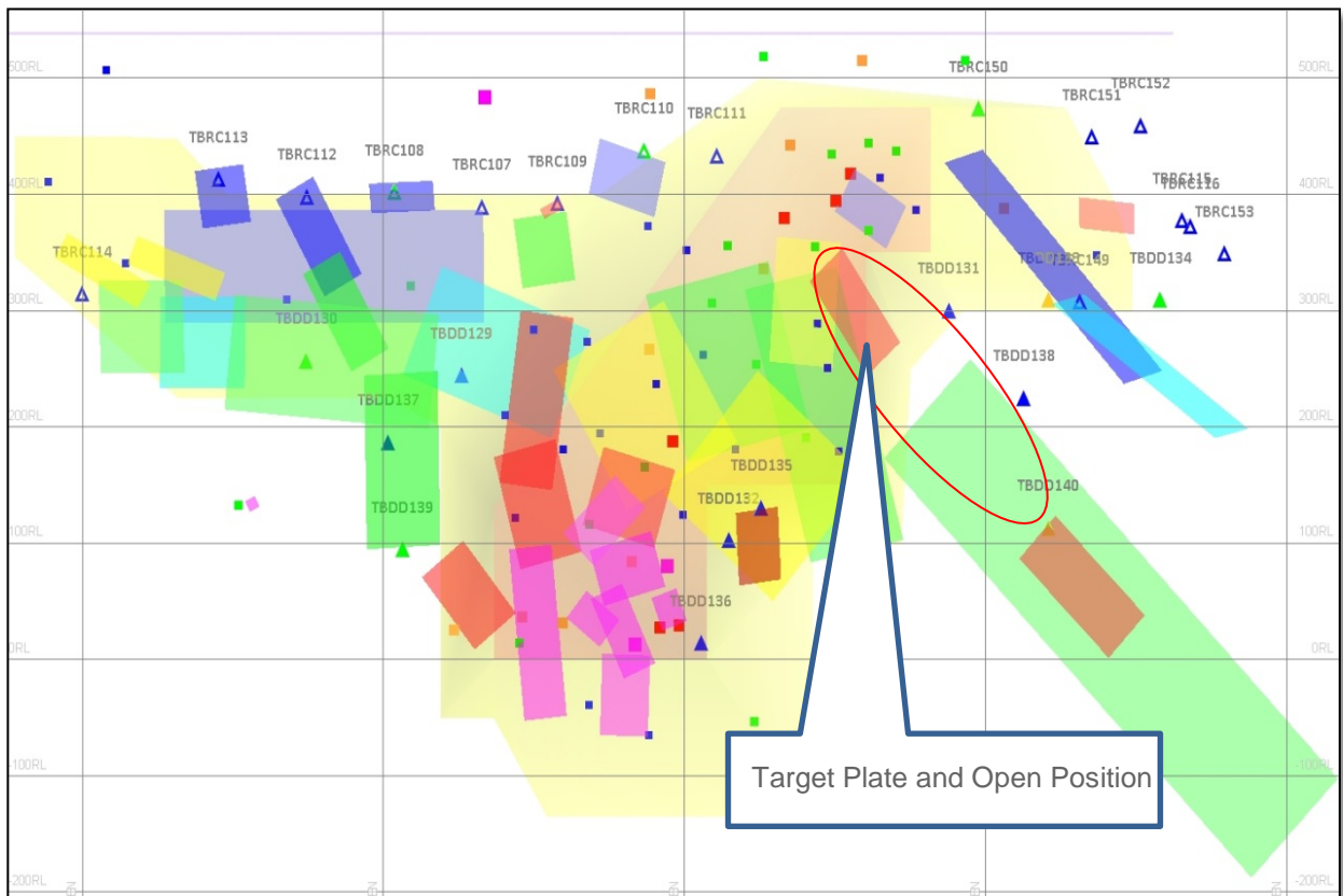
Figure 4: Rosie Long section with Ni%xm pierce points, circles pre 2012 drilling, triangles 2012 drilling (0-5 blue, 5-10 green, 10-15 orange, 15-20 red, >20 pink). EM plates coloured by conductivity thickness (0-1k light blue, 1k-5k blue, 6k-10k green, 11k-19k yellow, 20k-50k red, >50k pink)
