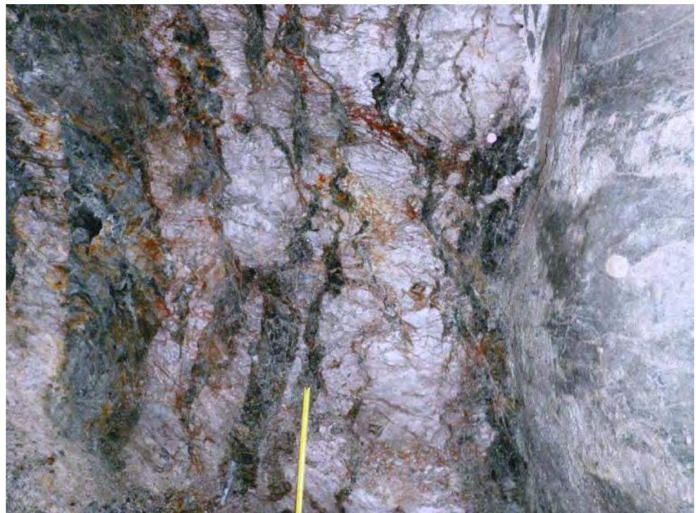
192mN Sublevel stope – 16m face West Reef. Highly silicified Porphyry dyke on RHS (Hanging Wall Shear).
