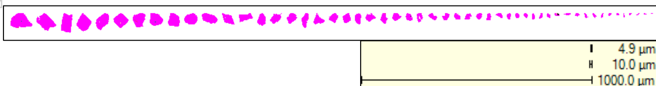
Figure 5 – QEMSCAN images of Zircon particles in sample composites from Los Conchaes showing grain size and degree of liberation (magenta colouring represents Zircon).
