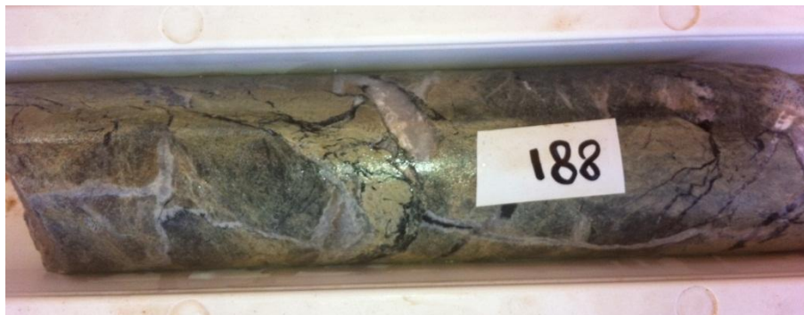
Figure 2. Photographs of MVPDH001 core displaying zones of variable intensities of quartz-carbonate veins and stringers and associated bleached sericite-chlorite alteration zones.
