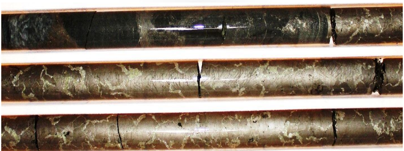
Figure 2. Photo of massive sulphides in hole SFRD0167, showing coarse grained pentlandite rims around pyrrhotite crystals.
