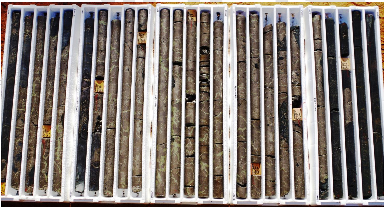
Figure 2. Photo of massive and breccia sulphides from SFRD0258, located 60 metres west of the Bollinger discovery hole.
