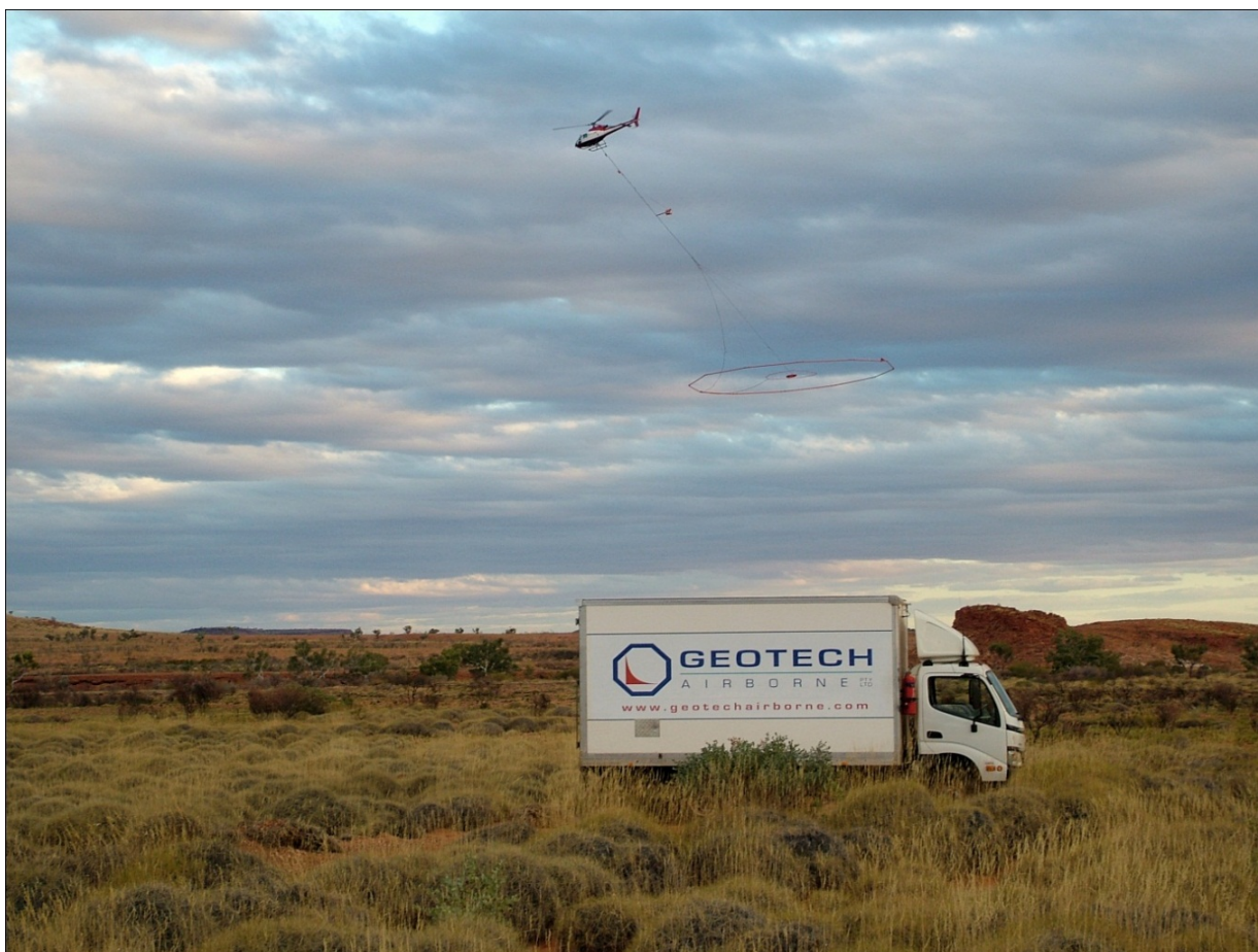
Figure 6: HeliVTEM survey (Photo courtesy of Geotech Airborne Pty Ltd)
