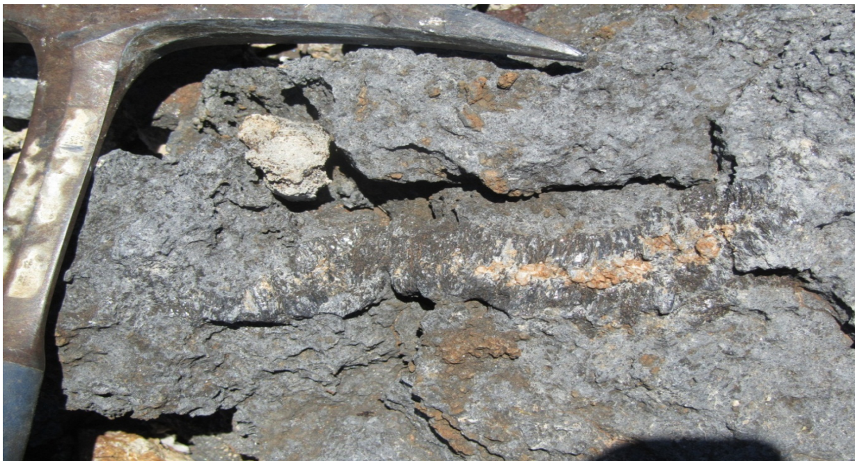
Figure 9: Coarse flake graphite vein hosted within high-grade, fine grained graphite rock.
