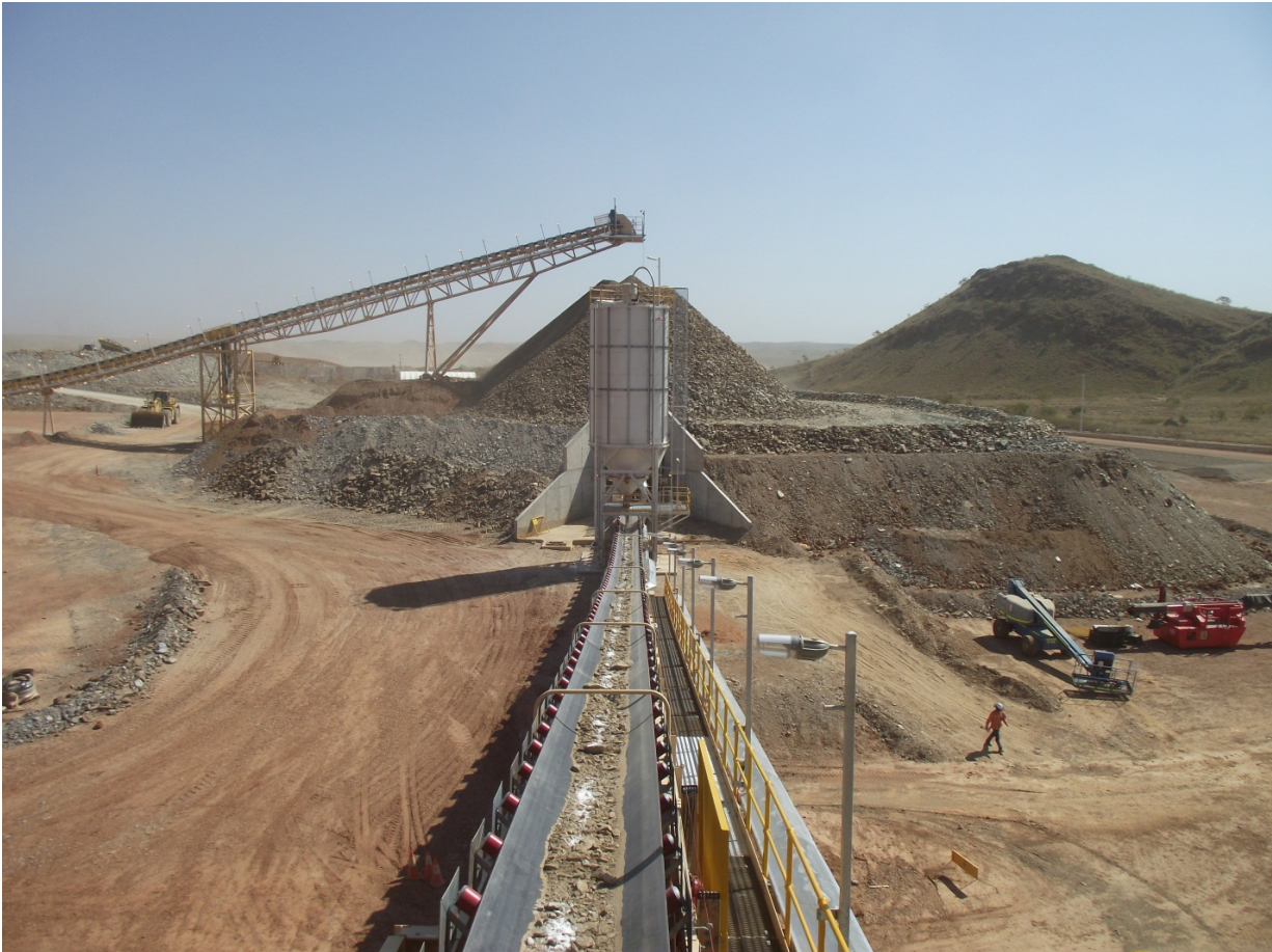
September 2012 - CV2 to Mill – Crushed Ore and Lime to Mill. Crushed Ore Stockpile-Background
